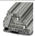
Multi-level terminal block, Connection method: Screw connection, Cross section: 0.14 mm² - 6 mm², AWG: 26 - 10, Width: 6.2 mm, Height: 60.1 mm, Color: gray, Mounting type: NS 35/7,5, NS 35/15
